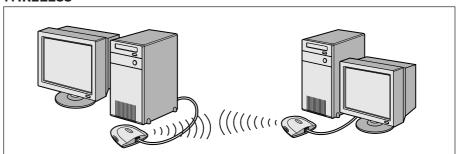
At each computer, you will need to install a WiFi wireless network adapter to be able to connect to another wireless network device. Examples are:
