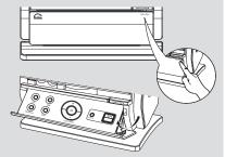
2 Insert the USB device's USB plug into the socket
