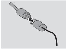
**Note:** If you are using a cable antenna system or an outdoor antenna, fit the antenna plug, instead of the wire antenna, to FM ANTENNA.
