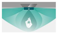
The basis of WaveFlector technology is a unique speaker system with three speakers, two side speakers and one centre speaker, located between two reflectors. The two side speakers are fired into extensively researched, calculated and defined reflectors so that sound, especially high frequencies, are reflected out into the room to the listener. Angling speakers into the reflector creates a wide and natural
