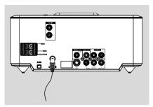
• Connect the supplied FM antenna to the FM (75  $\Omega$ ) jack. Extend the FM antenna and fix its end to the wall.
