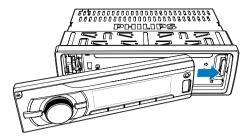
Press the left end of the front panel inwards until it is securely locked with a
