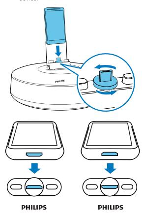
2 Slide the connector to the center of the device.
