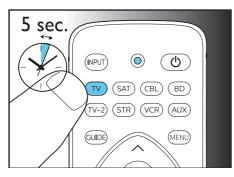
Point at your device with the universal remote. Then press and release U to start searching the code for your brand. A different infrared signal is sent every 2 seconds as the universal remote searches, indicated by a blue flash.
