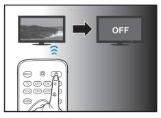
4 When the device is off, **immediately** press and release **OK** to save the code.The blue LED indicator will turn off.
