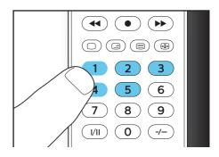
5 If the light is off, a valid code is saved. Otherwise, the light will flash six times, and then remains on for code re-entry.
