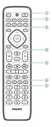
INPUT: select available source inputs (antenna, cable, etc.).
