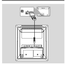
Connect the video and audio connectors of the supplied AV cable to the corresponding jacks on the SCART adapter, and then plug the adapter to the SCART jack of the TV.
