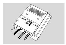
Align the side marked PRESS▼ of the stand to the slots at the bottom of the set.
