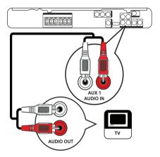
1 Connect the audio cables (not supplied) to the AUDIO IN-AUX1 jacks on the Home Theater System and the AUDIO output jacks on the TV.
