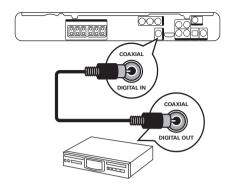
Connect a coaxial cable (not supplied) to the COAXIAL DIGITAL-IN jack on the Home Theater System and the COAXIAL/DIGITAL output jack on the device.
