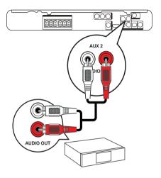
Connect the audio cables (not supplied) to the AUDIO IN-AUX2 jacks on the Home Theater System and the AUDIO output jacks on the device.
