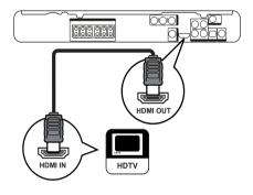
1 Connect an HDMI cable to the **HDMI**OUT jack on this Home Theater System and the HDMI input jack on the TV.
