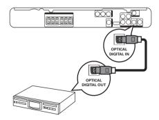
Connect an optical cable (not supplied) to the OPTICAL DIGITAL-IN jack on the Home Theater System and the OPTICAL/ SPDIF output jack on the device.
