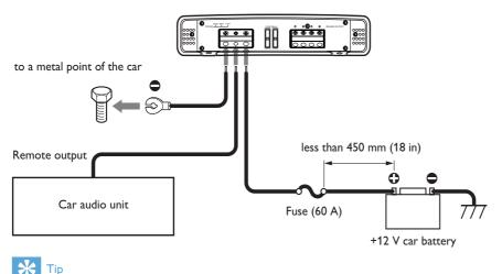
• If your car audio does not have remote output, connect the remote input terminal (REM) to the accessory power supply.
