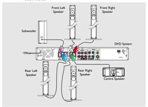
Connect the supplied speakers system using the fixed speaker cables by matching the colours of the sockets and speaker cables.
