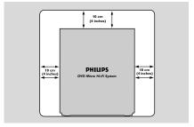
The ventilation should not be impeded by covering the ventilation openings with items, such as newspapers table-cloths, curtains, etc.
