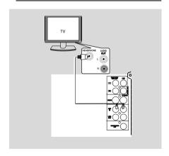
To listen to TV channels through this system, use the audio cables (white/red, not supplied) to connect AUX IN (L/R) jacks to the HEADPHONE jacks on the TV set (With a diameter 3.5mm stereo jack).
