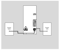
Connect the speaker wires to the SPEAKERS (FRONT) terminals, right speaker to "R" and left speaker to "L", coloured (marked) wire to "+" and black (unmarked) wire to "-". Fully insert the stripped portion of the speaker wire into the terminal as shown.
