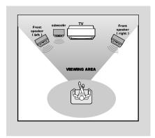
Place the front left and right speakers at equal distances from the TV set and at an angle of approximately 45 degrees from the listening position.
