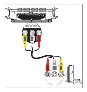
2 Connect the video input socket on the TV to the VIDEO OUT socket with the supplied yellow composite cable.
