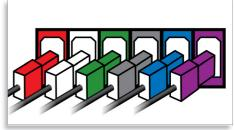
Colour-coded connectors provide a simple and user-friendly solution for connecting the speakers and subwoofer to the centre unit of the home entertainment system simply by plugging the connectors into the matching coloured interface at the rear of the centre unit.
