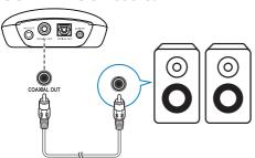
Connect a coaxial audio cable between
