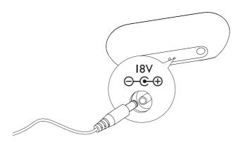
2 Connect one end of the AC power cord to the AC adaptor.
