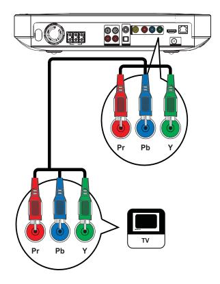
1 Connect the component video cable (not supplied) to the **Y Pb Pr** jacks on this Home Theater System and the COMPONENT VIDEO input jacks on the TV.
