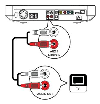
1 Connect the audio cables (not supplied) to the AUDIO IN-AUX1 jacks on this Home Theater System and the AUDIO output jacks on the TV.
