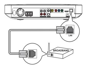
1 Connect the network cable (not supplied) to the LAN jack on this Home Theater System and the LAN jack on the broadband modem or router.
