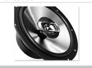
Inside the speaker, a diaphragm sits on top of a voice coil to produce a signal waveform once an input signal is received. It transforms the signal wave into a sound wave. Polypropylene is one of the lightest plastics ever invented and is great material for speaker diaphragms due to its weight, high strength, stiffness and tolerance for high temperatures. These polypropylene cones deliver high quality music by reacting to even the smallest sound signal to produce clear, vivid sound.
