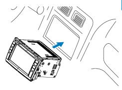
**6** Fix the unit onto the dashboard with screws.
