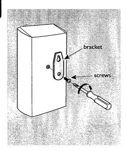
You can choose to hang the speakers on the wall. Attach the supplied bracket firmly to the rear of speakers using the supplied screws. Then mount a screw (not supplied) on the wall where the speaker is to be hung and hook the speaker securely onto the mounted screw.
