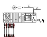
Connect the antenna and amplifier as illustrated, if applicable.
