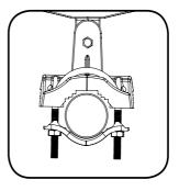
**3** Attach the assembly to the mast firmly.
