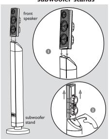
The connections between front speakers and DVD system are through the twin subwoofer stands.
