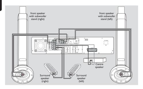
Connect the supplied speaker systems using the supplied speaker cables by matching the colours of the jacks and speaker cables. Fully insert the stripped portion of the speaker wire into the jacks.
