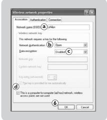
**5a** Fill in a Network name (SSID) you would like for your wireless network, for example: 'philips'.
