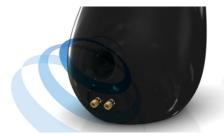
Bass-reflex acoustic load uses a bass pipe tuned to the acoustic volume of the speaker box, in order to reproduce deep bass from compact enclosures. The carefully designed profiled bass-pipe helps air flow and allows for deep and impactful bass, even at loud volumes while minimizing air turbulence that may cause distortion.
