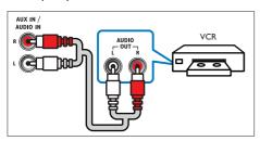
Using an analog cable, connect the AUX IN connector on your SoundStage to the AUDIO OUT connectors on the TV or other device.
