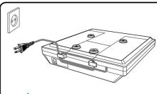
To prevent obstruction or danger, use the power cord posts to wrap the power cord so that excess cord does not hang down.
