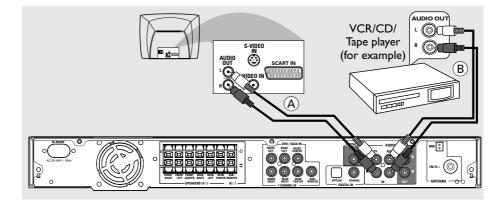
To hear the TV channels through this AV receiver, use the audio cables (white/red) to connect AUDIO IN-TV jacks to the corresponding AUDIO OUT jacks on the TV (see fig (A)).
