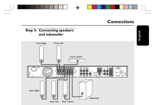
Connect the supplied speaker systems by matching the colours of the jacks and speaker cables. Fully insert the stripped portion of the speaker wire into the jacks.
