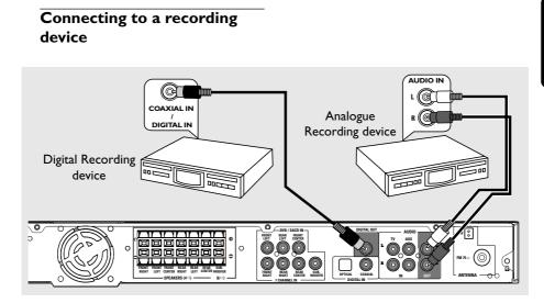
Connect the AV receiver's COAXIAL OUT jack to the DIGITAL (COAXIAL) IN jack on a digital recording device (DTS-Digital Theatre System compatible, with a Dolby Digital decoder, for example).
