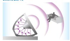
The carefully designed curved back cover creates a highly effective acoustic structure for sound reproduction. Its clean curve enforces the rigidity of the speaker cabinet, dramatically reducing internal resonance and eliminating the vibration and distortion of sound. You get to enjoy superb crystalclear sound in stunning looking speakers.
