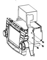
Slide the unit into the dashboard and fix it to the car with four screws.
