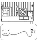
2 Stick the other end of the GPS antenna to a metal surface of the car.
