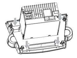
Fix the mounting brackets to the unit with screws (supplied by the car manufacturer).
