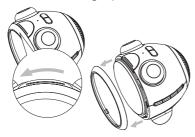
2 Place the ring to be installed onto the main unit.
