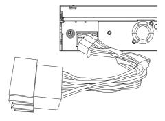
• If necessary, do the other connections. (See the last step in section **Connect wires: ISO connector**)
