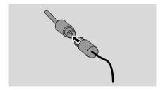
**Note:** If you are using a cable antenna system or an outdoor antenna, fit the antenna plug, instead of the wire antenna, to FM ANTENNA.
