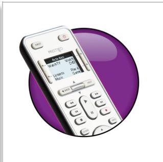
The remote features a 3.8-cm (96 x 64 pixels) LCD display. Less frequently used buttons are available via the display, so you can add your own buttons or remove the ones you do not need.
