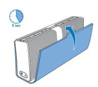
When you close the protective cover, the music play is muted. To unmute, open the cover within five seconds. When the protective cover is closed for more than five seconds, the speaker is switched off.
