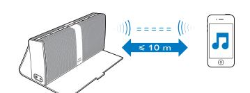
$\ensuremath{\mathsf{EN}}$  After successful connection, start music play on the Bluetooth device. The music streaming may be interrupted by obstacles between the device and P9, such as walls, or other devices nearby that operate in the same frequency.
