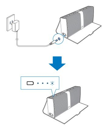
EN Charging ongoing: The four power LEDs light up white alternately. Charging complete: All four power LEDs light up white.
