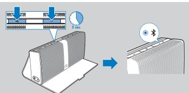
The amber light is on after the paired devices are cleared. Then, the white and blue light flashes alternately. You enter the pairing mode.
