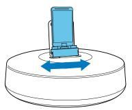
**3** Adjust the bumpers on both sides to stabilize the portable device.
