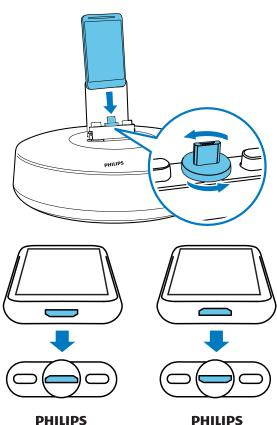
2 Slide the connector to the center of the device.
