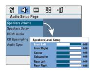
4 Use ◀▶ keys to set the volume level for each speaker (-6dB ~ +6dB) and press OK to confirm. 5 Use ▲▼ keys to highlight { Speakers Delay } and press ▶.
