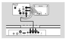
Use component video cables (red/blue/green - not supplied) to connect the DVD system's COMPONENT (Pr/Cr Pb/Cb Y) jacks to the corresponding Component video input jacks (or labeled as Y Pb/Cb Pr/Cr or YUV) on the TV.
