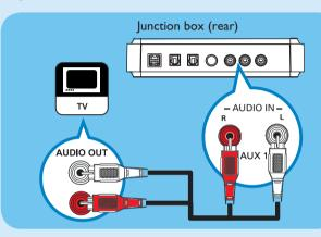
**Note** To listen to the audio output from this connection, press **AUX/DI /MP3 LINK** repeatedly until 'AUXI INPUT' is displayed on the display panel.
