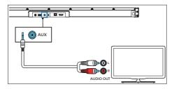
Use a RCA to 3.5mm audio cable to connect the TV's audio output sockets to the AUX socket on the unit.
