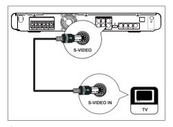
Connect a S-video cable (not supplied) from the VIDEO OUT-S-VIDEO socket on this unit to the S-Video input socket on your TV.
