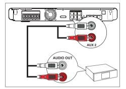
1 Connect an audio cable (not supplied) from the AUDIO IN-AUX2 sockets on this unit to the AUDIO OUT sockets on the device.
