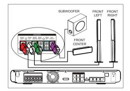
Connect the centre, front left, front right speakers and subwoofer to the matching sockets on this unit.
