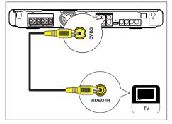
Connect a composite video cable (yellow supplied) from the VIDEO OUT-CVBS socket on this unit to the video input socket on your TV.
