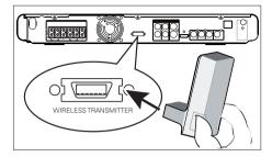
1 Connect the wireless transmitter to the WIRELESS TRANSMITTER socket on this unit.
