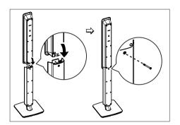
1 Attach the speakers to the speaker stands and secure the position with screws.
