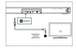
• Use an RCA to 3.5mm audio cable to connect the TV's audio output sockets to the AUX socket on the unit.
