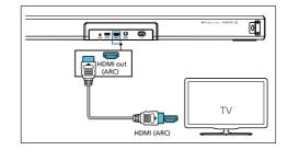
2 Using a High Speed HDMI cable, connect the HDMI ARC connector on your soundbar to the HDMI ARC connector on the TV.
