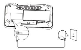
2 Connect the other end of the AC adaptor to the wall outlet.
