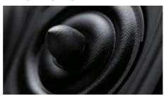
Philips docking speaker features a ring radiator tweeter - a high quality transducer used in Hi-
