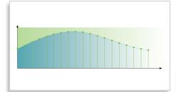
192 kHz sampling enables you to have an accurate representation of the original sound curves. Together with a 24-bit resolution, more information is captured from the original analogue sound wave form, giving a much richer audio reproduction.
