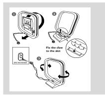
Position the antenna as far as possible from a TV, VCR or other radiation source.
