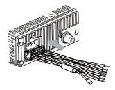
2 Connect the other end of the supplied standard connector to the unit.
