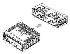
Install the sleeve into the dashboard and bend the tabs outward to fix the sleeve.
