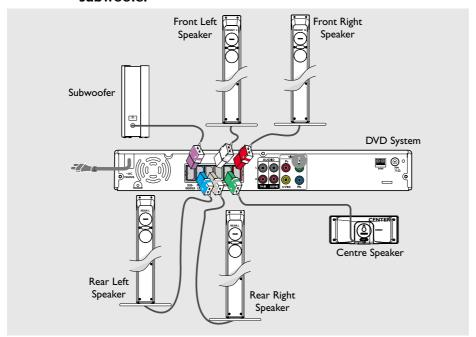
Connect the supplied speakers system using the fixed speaker cables by matching the colours of the sockets and speaker cables.
