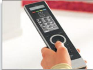
One-touch control allows you to perform multiple commands with one press of a button via a macro. A macro combines a string of pre-programmed commands under one single button. Therefore, it simply takes one button press to execute a series of functions.
